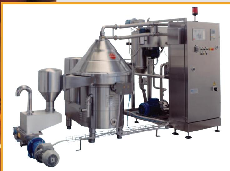
Self-cleaning separator with hydrocyclon for fruit juices clarification
