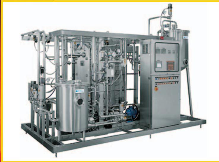
**Plates egg pasteurizing unit with degaser**
