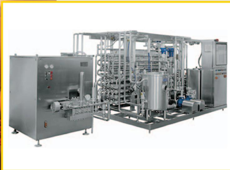
**Tubular egg pasteurizing unit with homogenizer**
